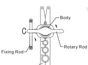
Open the tube expander bar and put the tube into the right place according to its required dimension.
